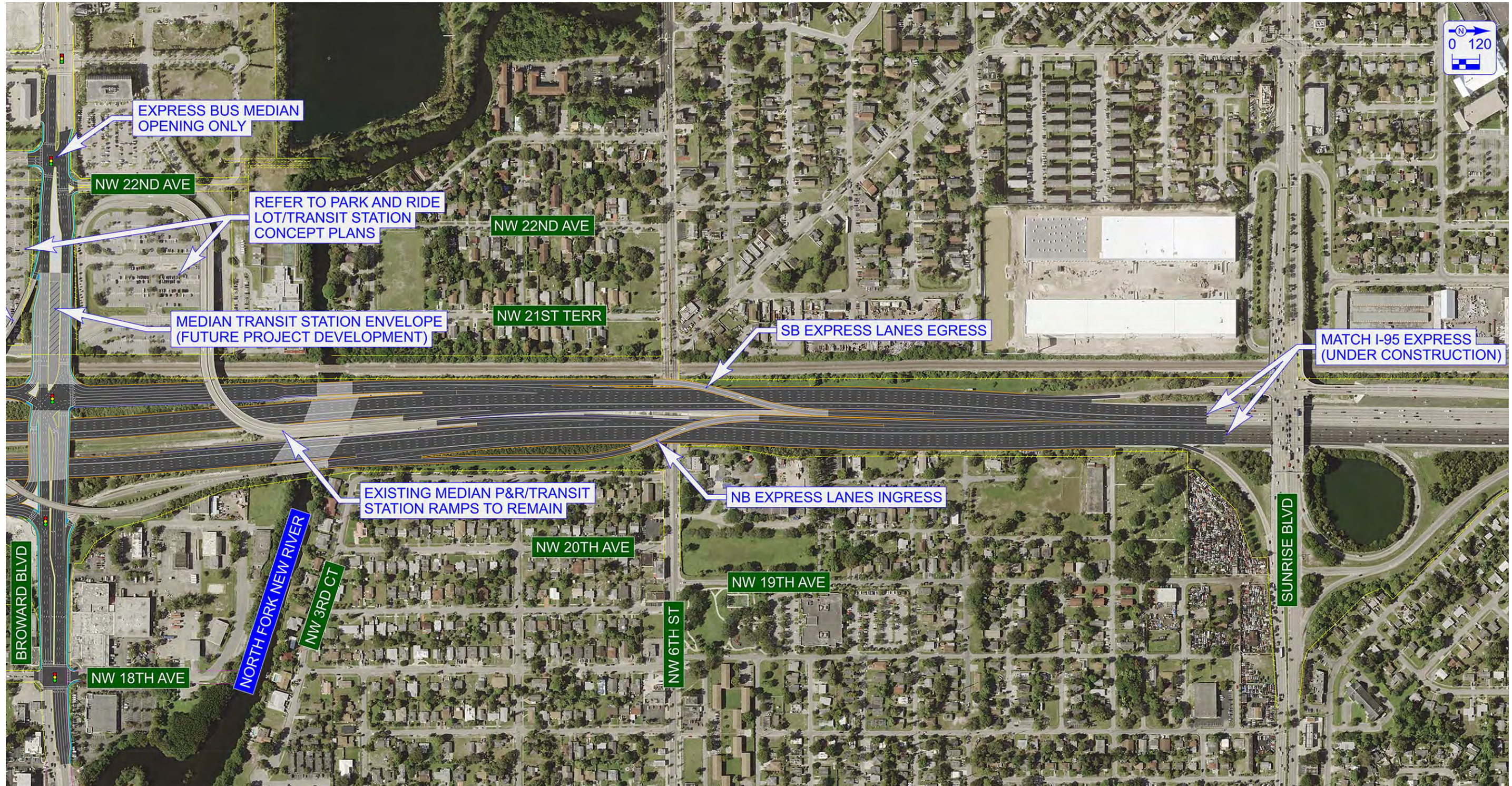
Figure E-3 | Mainline Build Alternative – 95 Express Ingress-Egress Connections with Broward Boulevard Interchange
