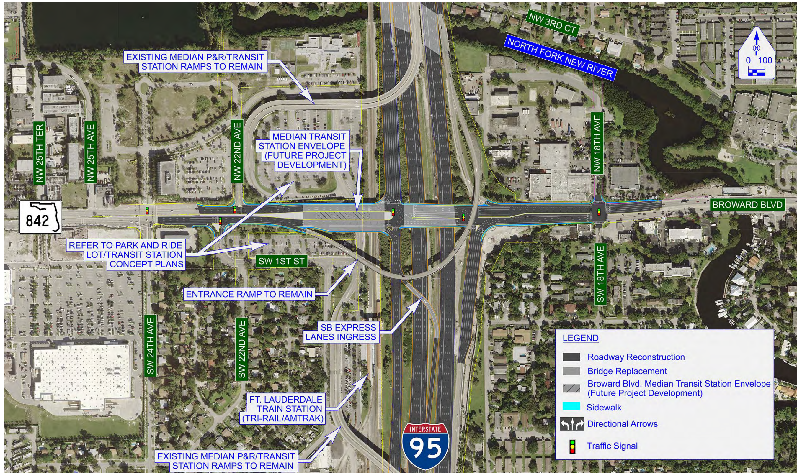
Figure E-4 | Interchange Alternative 1 – Tight Diamond
