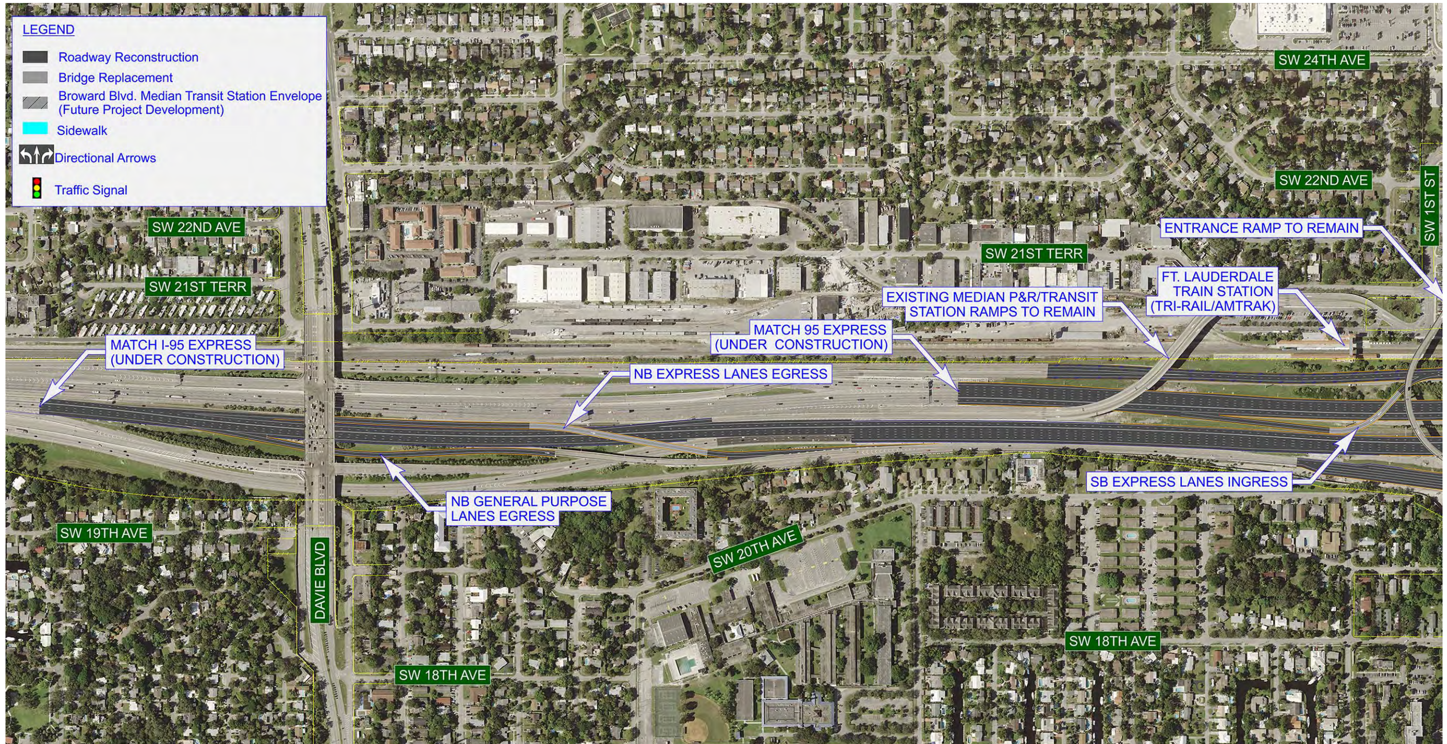
Figure E-2 | Mainline Build Alternative – 95 Express Ingress-Egress Connections with Broward Boulevard Interchange
